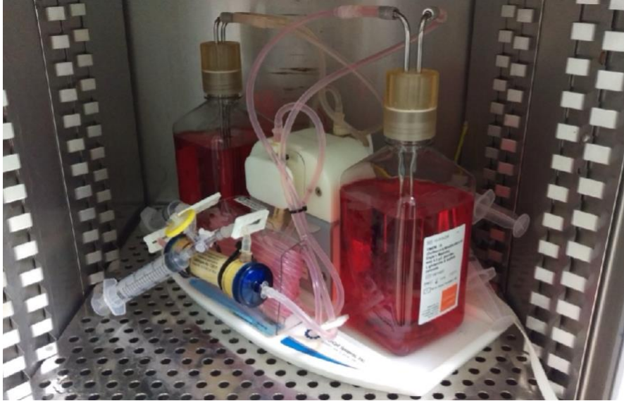
Figure 9: The hollow fiber bioreactor fits inside a standard CO 2 incubator. Temperature and gas are controlled by the conditions of the incubator. Reduced handling time and no cell passaging reduces the time the cells are outside of the incubator.
