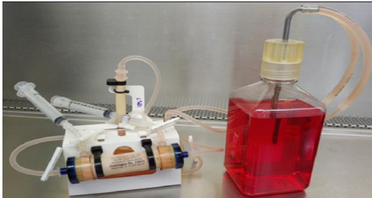
Figure 4: The FiberCell hollow fiber bioreactor is a completely closed system providing protection for the cells from microbial contamination and protection for the operator when working with infectious pathog
